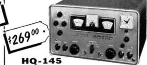
Brand-new general-coverage receiver! 540 KCS to 30.0 MCS. Dual conversion. Adjustable 60 db slot filter. Crystal filter. 11-tube superheter-odyne with automatic noise limiter.
