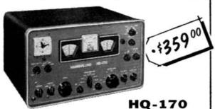
Best for the amateur at any price! Dual and triple conversion 17-tube superheterodyne with automatic noise limiter. 60 db slot filter. Separate vernier tuning. Selectable sideband. Tuned IF amplifier. Crystal calibrator.
