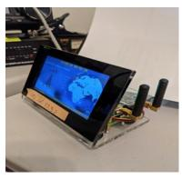
A duplex hotspot can also be used to create your own personal repeater. Since the power output is in the milliwatt range, it will only serve over a short distance. We won't pursue the repeater application in this document.
