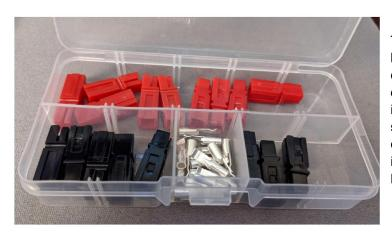
The middle section of this box holds the metal electrical connectors that are crimped on the electric cables before insertion into the Anderson shells. These metal connectors are then inserted into the back of the Red and Black shells.
