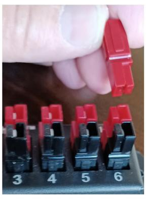
To be sure you have each pair of APs correctly positioned, take an empty pair and insert them into the target terminal strip or cable as you begin your project.
