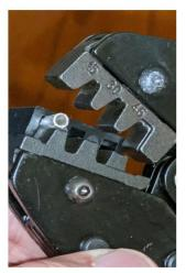
This Crimp Wrench has slots marked for each of the three-sized electrical connectors. The tongue is placed into the Crimp Wrench with the curved end facing down. Once the curved end is properly positioned within the wrench, partially compress the wrench to keep the connector from rotating while the appropriate wire gauge and length of center-conductor are inserted into the barrel for crimping.
