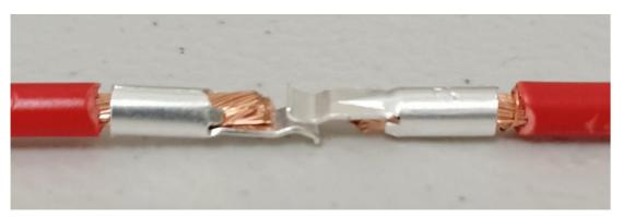
When plugging one AP into another, several problems can occur if the stripping of the wires exceeds % of an inch. On the left side, note the length of the center-conductor places it very close to interfering with the CONTACT POINTS between the two connectors.
