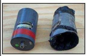
A few months ago the 146.610 repeater went off the air due to a lighting strike to the WROK tower. Being that the tower is a live tower a device called an isocoupler is used to isolate the repeater from the tower. The picture on the left is what a good one looks like, the one on the right is why the repeater was down for about 3 days. Luckily the station engineer for WROK had a spare one laying around so Herb, K9AMJ, was able to replace it at no expense to the club.
