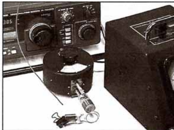
Figure 6—A calibrated receiver is used to monitor the dip meter's exact frequency while a crystal is "dipped."
