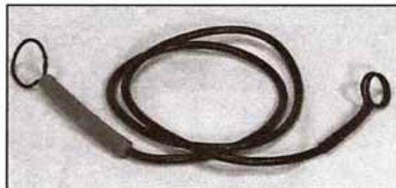
Figure 3—A coaxial cable "link" with a coil at each end is used to extend the reach of the dip meter's plug-in coil.
