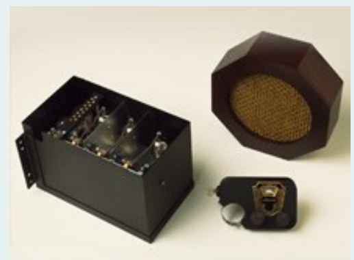
This reproduction of Motorola's first car radio, 1930's model 5T71, included (left to right) a radio receiver, tuning control and speaker.
