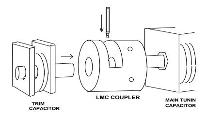
Even though I benefited from Dave Larsen's skill in machining, I believe one could make such an LMC with a drill press, a hack saw, and a 6/32 tap set. Many of us have such tools on our work bench.
