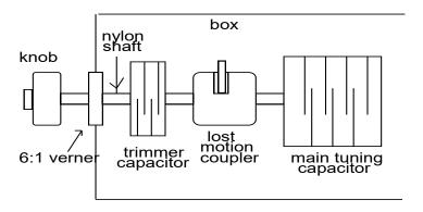
Dave Larsen N9ZXL made the coupler for me from a 3/4" diameter piece of round brass stock about 3/4 inch long. He drilled a 1/4" hole down the center and milled a cross-wise (transverse) notch half way down to the drilled hole. After that, a few drilled holes for set screws finished the job.
