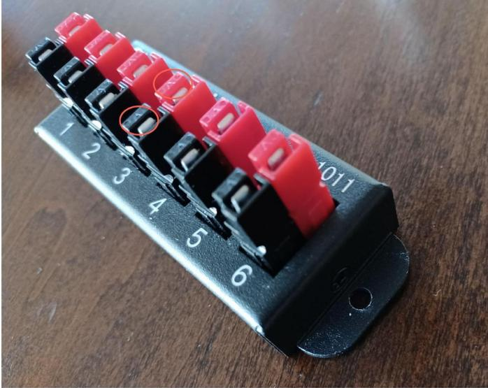
This commercial terminal block is made up of 6 sets of Anderson Powerpoles. One pair of cables plugged into any of those 6 will carry the 12 volt Power Supply to all of the remaining 5 terminals. Each additional pair of Anderson cables plugged into these available terminals will then carry that 12 volt power to another piece of equipment like a radio or tuner.
