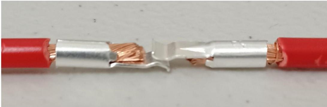
When plugging one AP into another, several problems can occur if the stripping of the wires exceeds  $\frac{3}{8}$  of an inch. On the left side, note the length of the center-conductor places it very close to interfering with the CONTACT POINTS between the two connectors.
