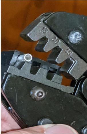
This Crimp Wrench has slots marked for each of the three-sized electrical connectors. The tongue is placed into the Crimp Wrench with the curved end facing down. Once the curved end is properly positioned within the wrench, partially compress the wrench to keep the connector from rotating while the appropriate wire gauge and length of center-conductor are inserted into the barrel for crimping.
